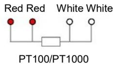
Connections are made via the 2-way terminal block. Connections for thermistor, platinum and nickel sensing elements are polarity independent.
