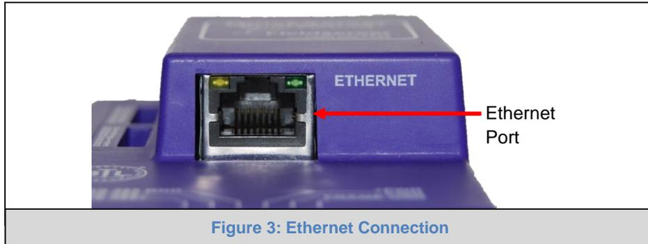
Figure 3: Ethernet Connection
