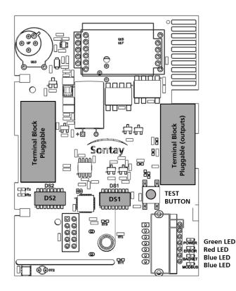
When using the digital input as a VFC, the VFC contacts should be connected across the DI terminal and the common 0v terminal, i.e. active low.
