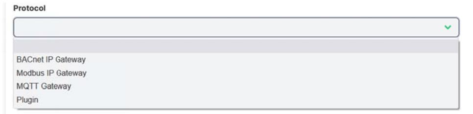
The screenshot shows a dropdown menu titled "Protocol" with a green checkmark icon on the right. The menu is open, showing four options: "BACnet IP Gateway", "Modbus IP Gateway", "MQTT Gateway", and "Plugin".
