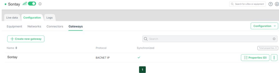
Click on the 'Properties' button to the right of the BACnet IP gateway, then click on the '+ Add Property button'. A list of LoRa device properties are then shown. Tick the properties you want to see as BACnet objects.
