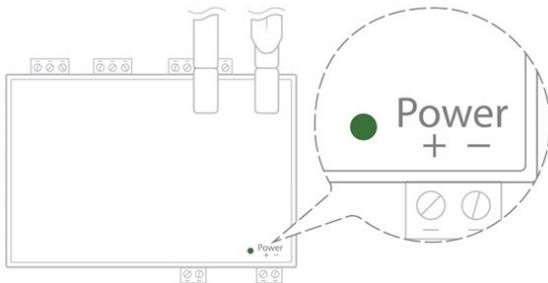
The Bridge is protected against overvoltage, undervoltage, overcurrent from the power supply with indication by LED: green LED when the power supply is compatible, red LED if it is not suitable. Change the power supply to avoid damaging the Bridge.
