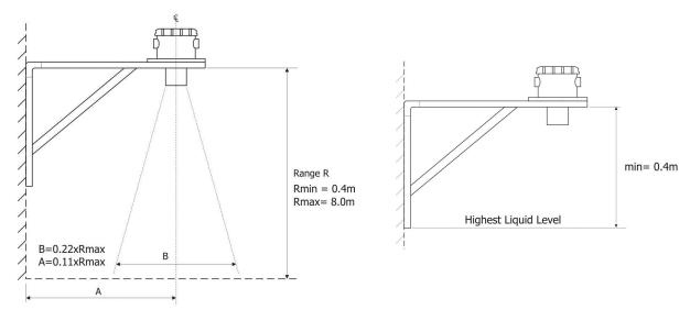
The LS-UT has a 'dead band' of 0.4m from its sensor face. Ensure that the highest liquid level does not enter this 'dead band'. Liquid closer than 0.4m will result in false measurements, which may appear as distances several times the real liquid level.
